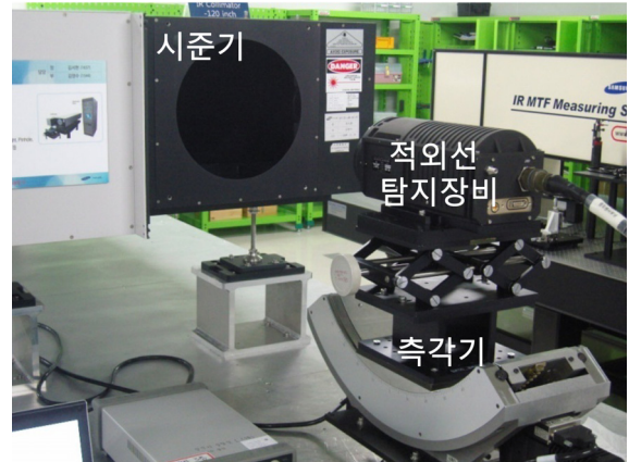
FIG. 3. Configuration of the Minimum Detectable Irradiance(MDI) measurement.
