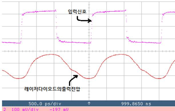
FIG. 4. Measured input and output waveforms of the optical transmitter at 1Gbps.
