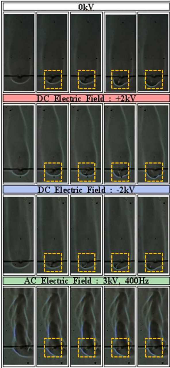
Fig. 13 Instantaneous images of wire flame for fixed exposure
