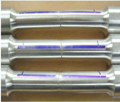
Fig. 5 Tensile specimens after testing
