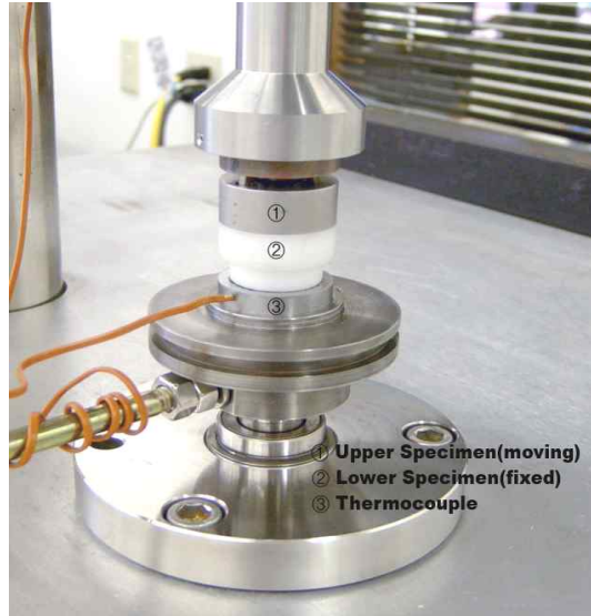
Fig. 1 Schematic diagram of disc on disc configuration for nylon
