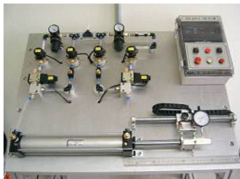
Fig. 1 Photograph of the position control system of a pneumatic cylinder
