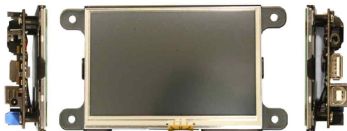
Fig. 10 The photograph of the embedded controller with touch panel
