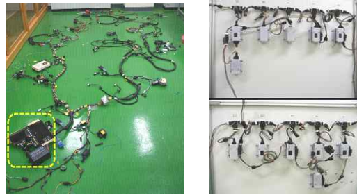
(a) Original wiring (b) Developed wiring Fig. 13 The photographs of the original and newly developed wiring harnesses for comparison
