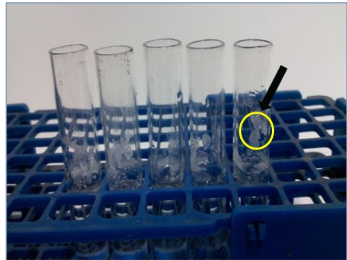
[Fig. 3] Crystal formed at the CO 2 absorber during AT 4 measurement.
