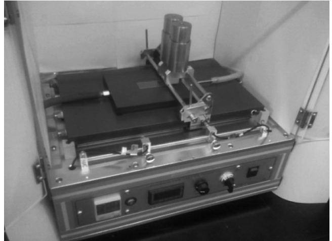
Figure 2. Photo of a bar coater type coating apparatus used in this study.
