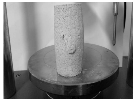
Fig. 7. Unconfined compression test for artificial soil specimen.
