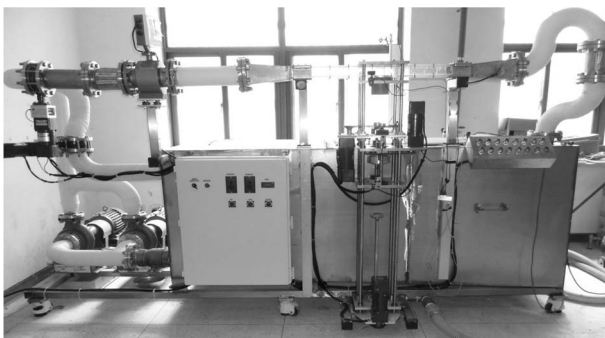
Fig. 4. Improved hydraulic resistance measurement apparatus of Chonnam National University.
