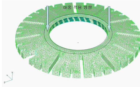
Fig. 4 Meshing and direction of force
