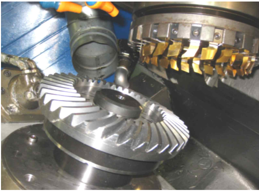
Fig. 1 Tooth profile machining of the ring gear
