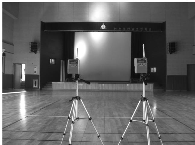
**Figure 2. Air sampler for VOCs and formaldehyde.**
