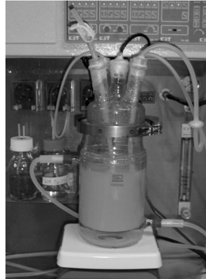
Figure 1. Experimental set-up of pH control bioreactor.
