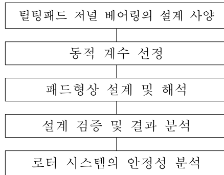
Fig. 15 Design procedures of tilting pad journal bearing
