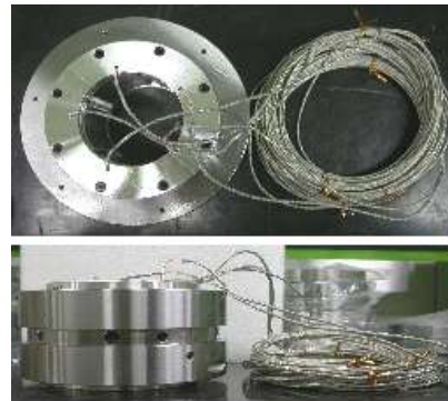
Fig. 11 Prototype of 5 pad tilting pad journal bearing for experiment
