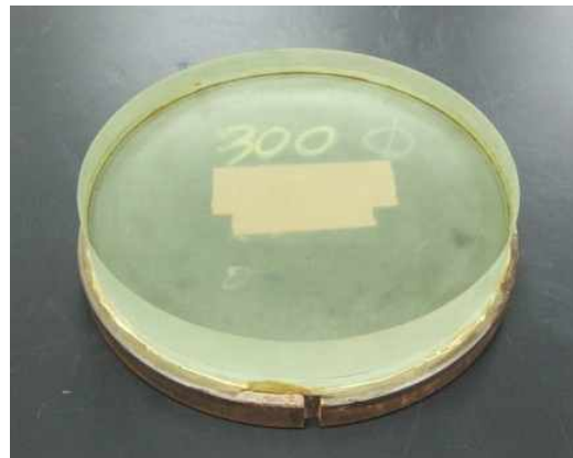
Fig. 8 Photograph of the test piece with aspheric surface
