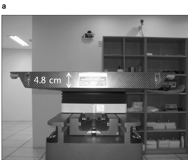
Fig. 2. A side view of couch top (a) and Schematic overview of thickness variation to incident angle (geometric model) (b).
