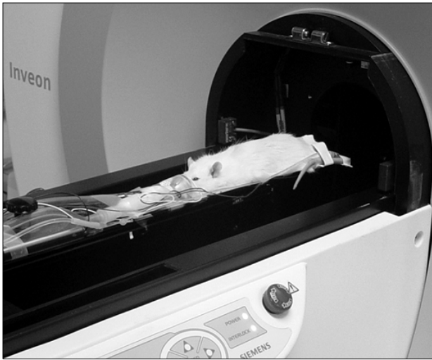
Fig. 1. Small animal Inveon™ PET scanner (Siemens Preclinical Solutions, Knoxville, TN, USA) using physiological monitoring and triggering system (BioVet, m2m Imag. Corp).
