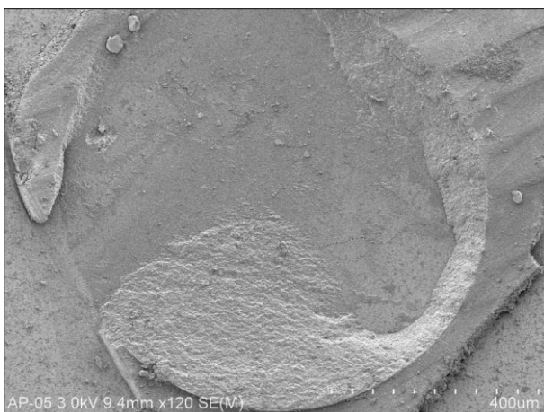
Figure 5. Representative mixed failure to enamel surface in AP group ( \times 120 ).
