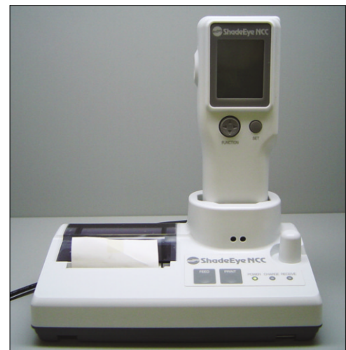
Fig. 2. Dental colorimeter (ShadeEye NCC® Chroma Meter, Shofu Dental).
