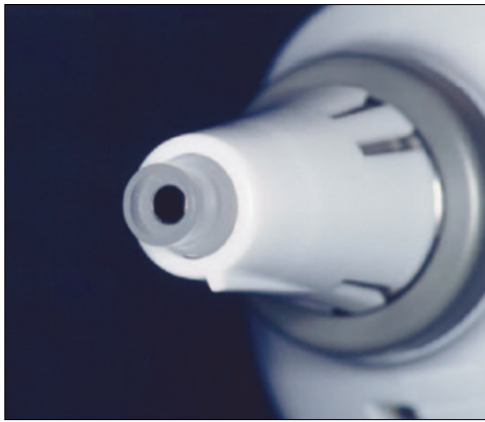
Fig. 3. Touch probe aperture of ShadeEye NCC® Chroma Meter.
