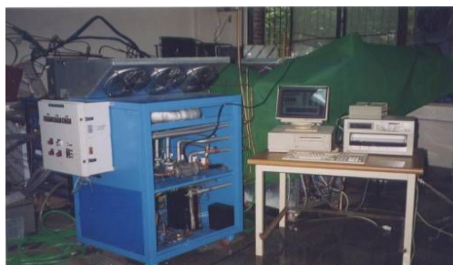
Figure 5. Experimental equipment composed of the PC-based automatic data acquisition unit and the heat pump system (2.2 kW).
