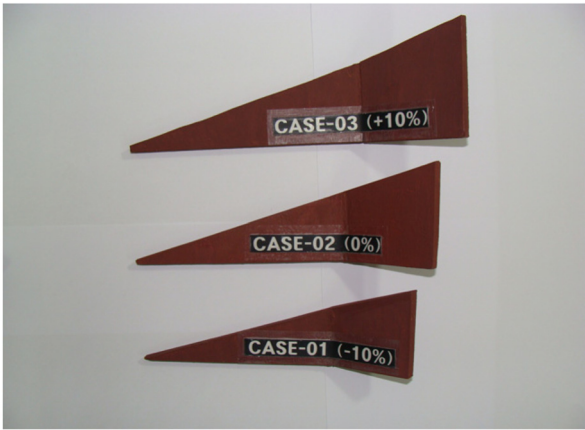
Fig. 6 Designed model skegs
