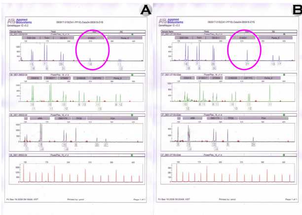
Fig. 1. Electropherograms showing results of DNA typing. STR profiles were analyzed on an ABI PRISM® 3100 Genetic Analyzer after co-amplification of thirteen STRs plus the Amelogenin with PowerPlex® 16 System Kit. Profile show that the D18S51 locus is homozygous (16, 16 and 21, 21) genotype.
