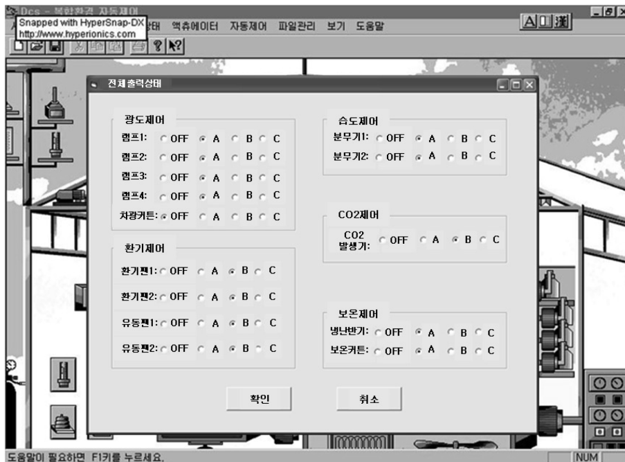
Fig. 7. Overall control screen in automatic control system.
