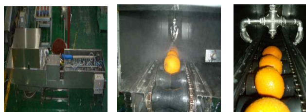
Fig. 1. Surface washing system of yuja .
