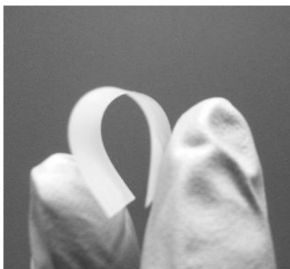
Figure 3. Photographs of the flexible SPT film containing 3 wt% PVA. Film size : 50 mm × 25 mm.
