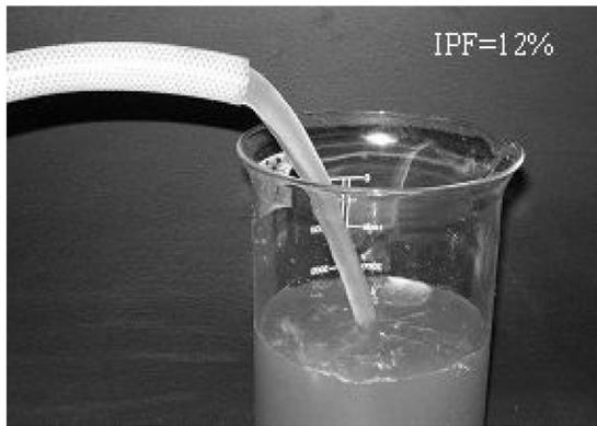
Fig. 1. Fluidity of the ice slurry.
