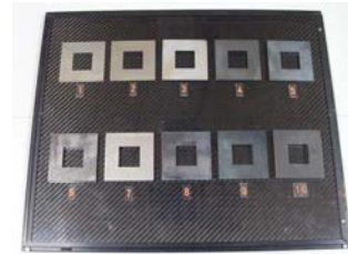
Fig. 4. A square iron plate made to measure sharpness (Size : 70 mm × 70 mm, Thickness : 1~10 mm)
