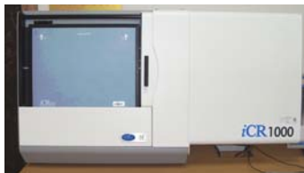
Fig. 1. CR equipment to measure the number of dark spots of image plates.
