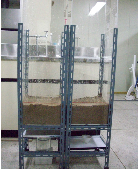
Fig 2. The device for artificial rain and paraquat elution
