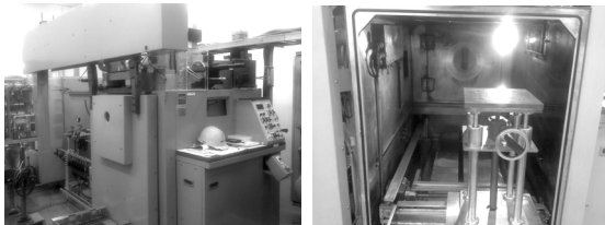
Fig. 3 Electron beam welding system used
