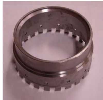
Fig. 1 Annulus gear sample having hollow geometry
