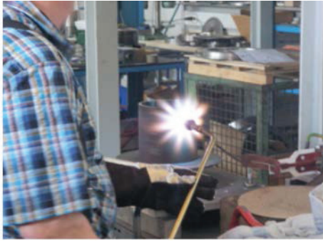
Fig.13 Flow forming experiment for annulus gear
