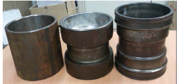
Fig.14 Rollers set-up for annulus gear forming
