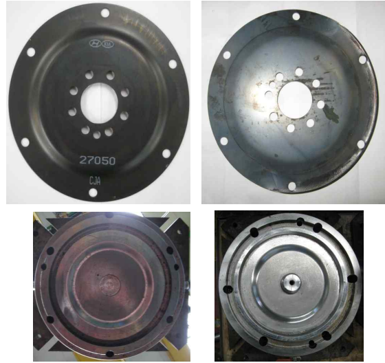
Fig. 8 Shapes of actual drive plate(above left) and press-quenched drive plate(above right), and dies for press quenching(below)
