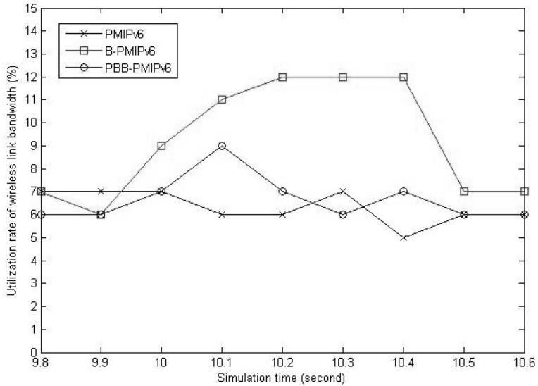
Fig. 7. Comparison of resource utilizations over a wireless link
