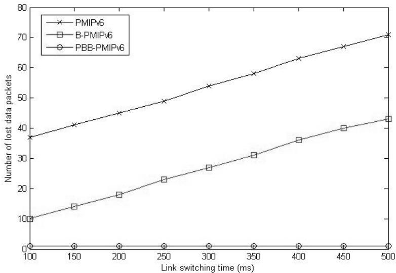
Fig. 9. Comparison of packet losses during handover
