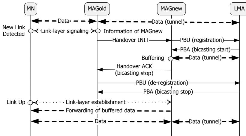
Fig. 4. Proposed PBB-PMIP scheme
