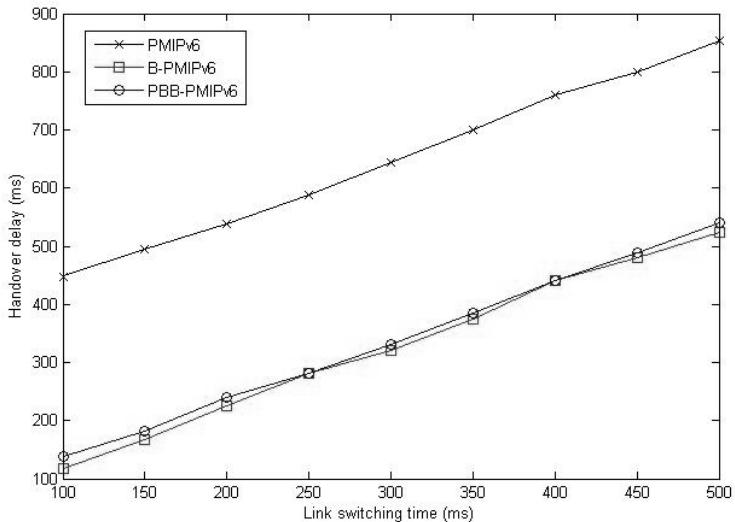
Fig. 8. Comparison of handover delays during handover
