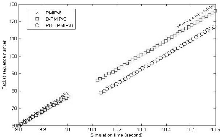
Fig. 6. Traces of data packets transmitted during simulation
