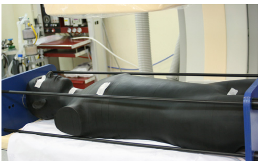
Fig. 3. Rando phantom skin TLD chip attach
