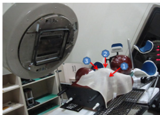
Fig. 6. The experiment which uses the linear accelerator. ① 1.5 cm point from RAO beam CA, ② The farthest point from both beam, ③ 1.5 cm point from LPO beam CA
