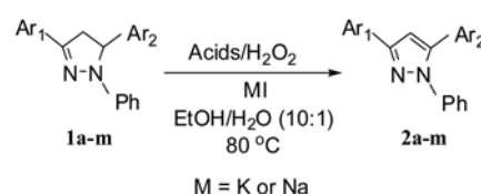
Scheme 1. Aromatization of 1,3,5-trisubstituted-2-pyrazoline.
