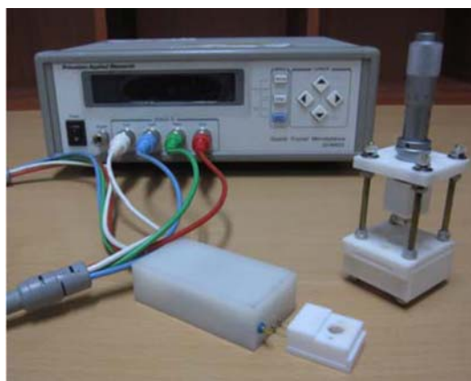
Figure 1. Apparatus setup for QCM measurements.
