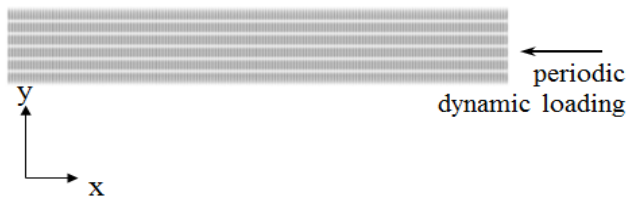
Fig. 7 Simple FE shell model with a periodic loading.
