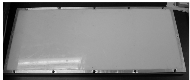
(b) Photo of a typical compliant coating test plate.
