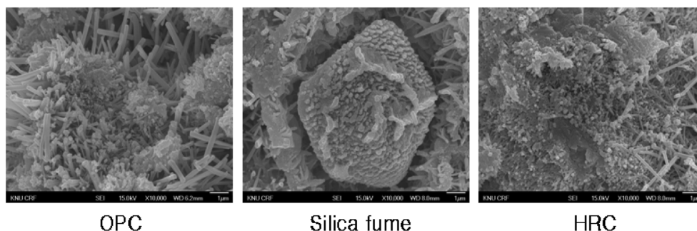
Fig. 14. SEM of 3 day OPC, SF, and HRC.
