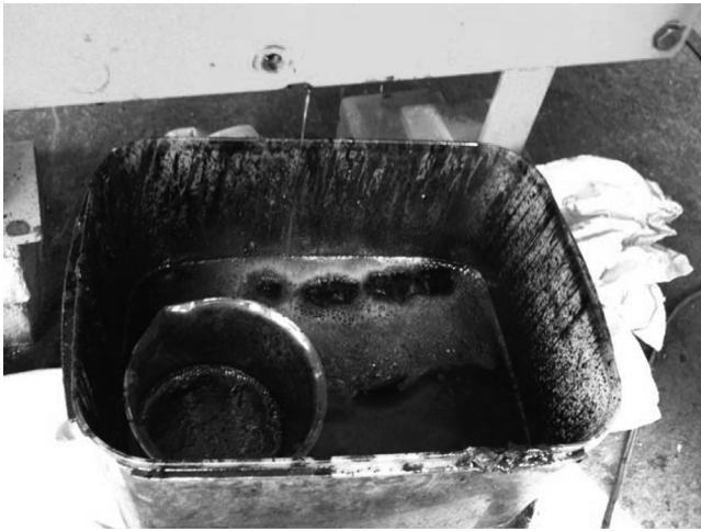
Photo 2 Collection of condensed water vapor and tar from filter box
