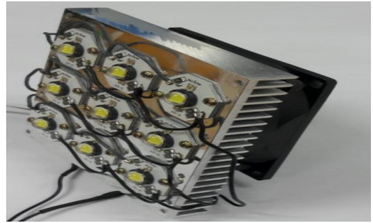
Figure 1: LED cooling system
