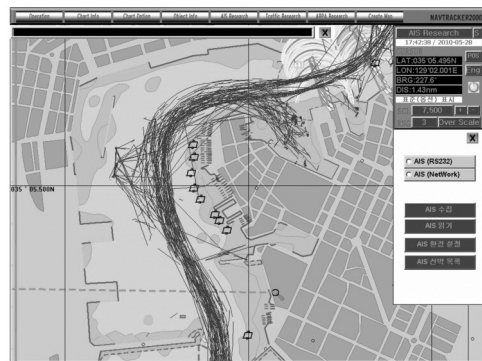
Fig. 4. Vessel data analysis module for the marine traffic survey system.
