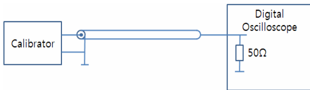
Fig. 4. Alternative method to estimate the PD calibrator
