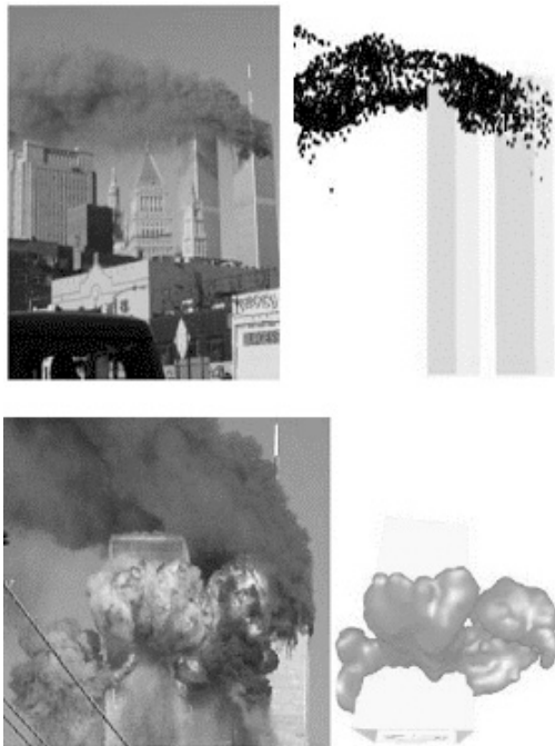
Fig. 6 Comparison of the real fire(WTC; World Trade Center) and FDS
