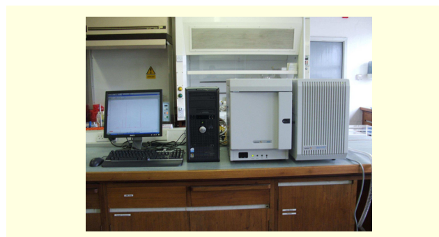
Fig. 1. GC-MS apparatus operated in the electron-ionisation mode used for analysis. Bacteria headspace sample analysis and SPME concentration was performed with Supelco fibers. Controls were carried out using agar media blanks.
