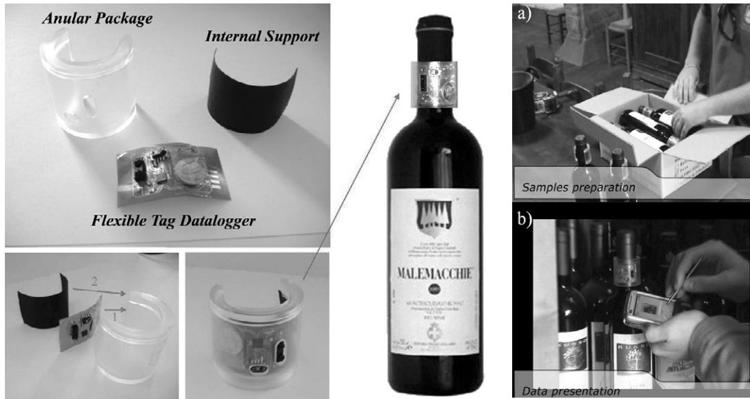
Fig. 8. FTD for wine chain logistics: packaging, assembling, and application on a wine bottle (a) A moment of the sample preparation. (b) FTD data reading by using a HP iPAQ rw6815 Smartphone equipped with reading software. (Mattoli et al., 2009)
