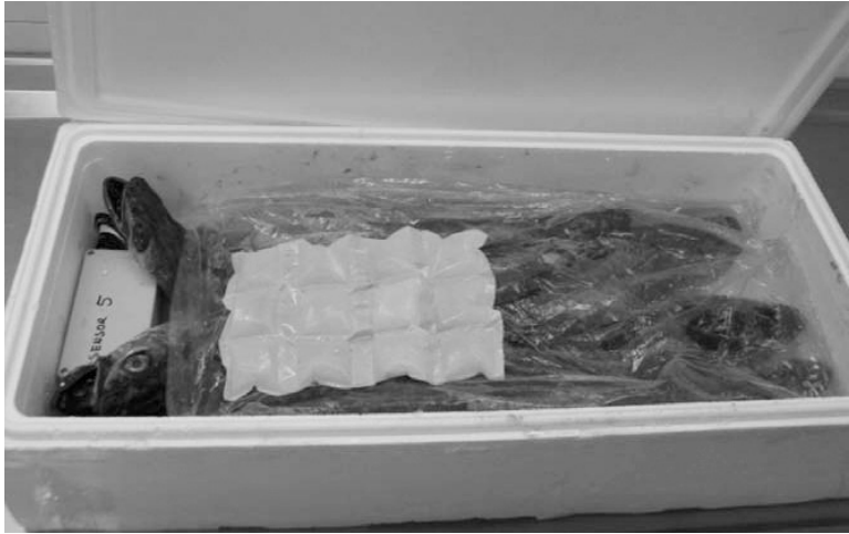
Fig. 6. Smart tag placed inside a polystyrene box with the fish and the cooling gels. (Abad et al., 2009)
