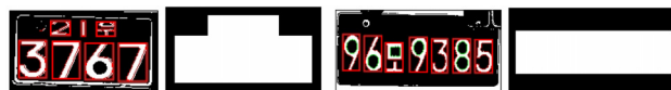
FIG. 8. Two reference images: Connected components of characters and their segmented inner area and outer area.
