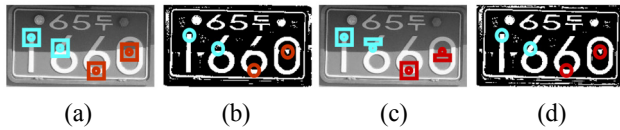
FIG. 5. Comparison of binarized results: (a) fixed windows; (b) binarized image by Niblack's method; (c) adaptive windows; (d) binarized image by the proposed method.
