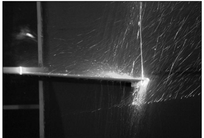
Fig.7. Image of rainwater penetration paths
