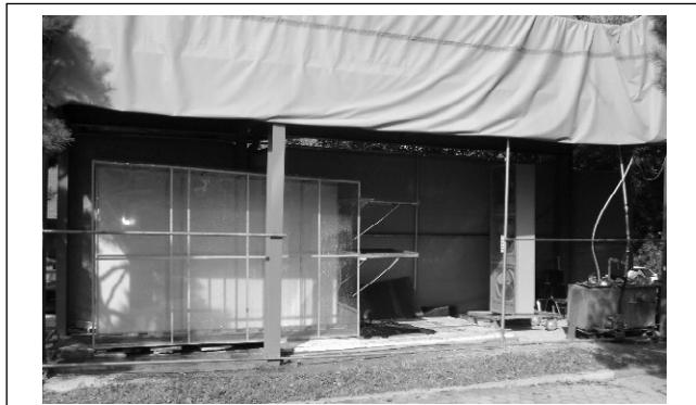
Fig.3. Photo of experimental setup for rain penetration of windows
