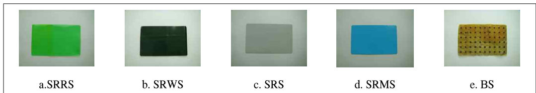
Figure 1. Selected materials (SRRS; synthetic resin system root barrier sheet, SRWS; synthetic resin system root barrier · waterproof sheet, SRS; synthetic rubber system root barrier sheet, SRMS; synthetic rubber system membrane root barrier sheet, BS; barrier sheet).
