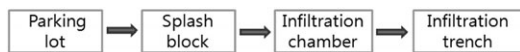
Figure 2. Parking lot runoff through the infiltration chamber & infiltration trench at 1st housing complex completed in 2006
